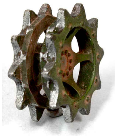
Look of the teeth polished by the rubbing of the track.
